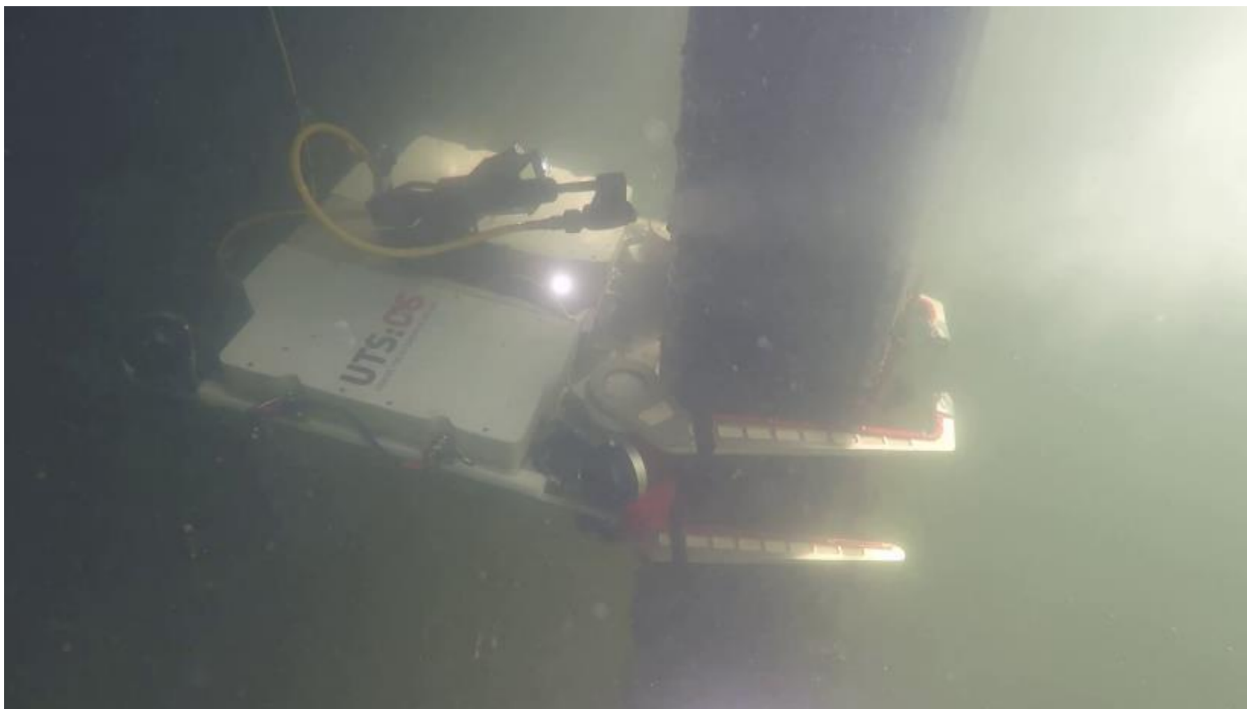
Figure 8: Underwater robots developed in Sydney for cleaning and inspection of underwater objects (UTS, 2021)
