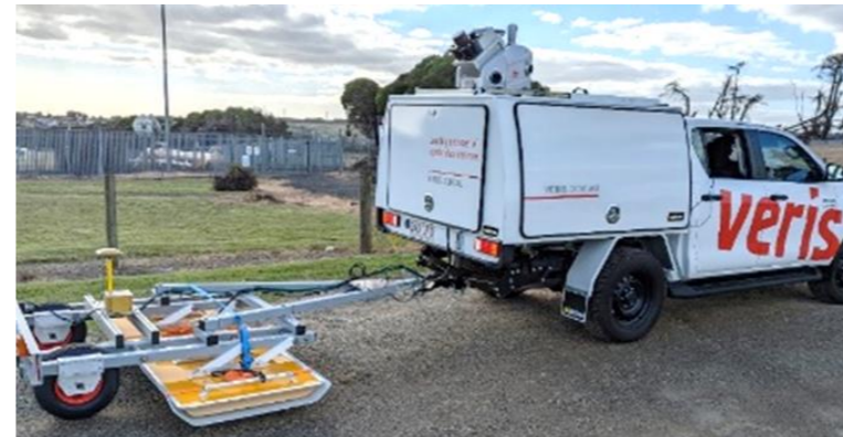
Figure 9: Overview dashboard of GPR scanning and advanced image processing of subsurface road (above) and vehicle-towed 3D GPR unit (right) (Veris, 2024)
