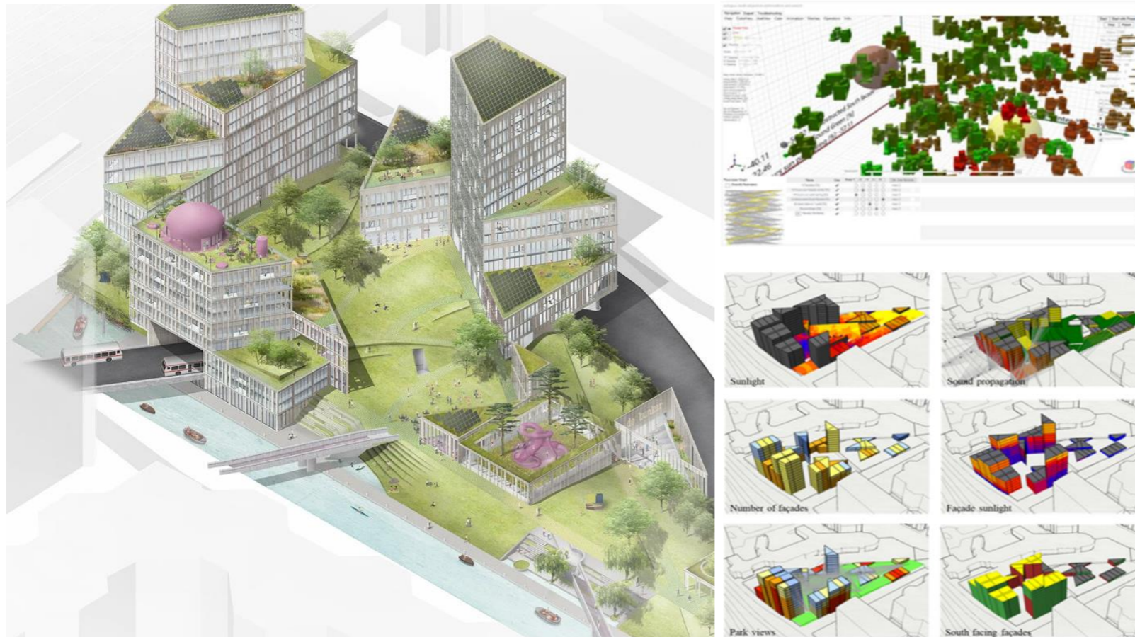
Figure 7: Parametric design applied to Smakkelaarspark redevelopment used to optimise design for noise, sun exposure and energy generation (Arup, 2024b).
