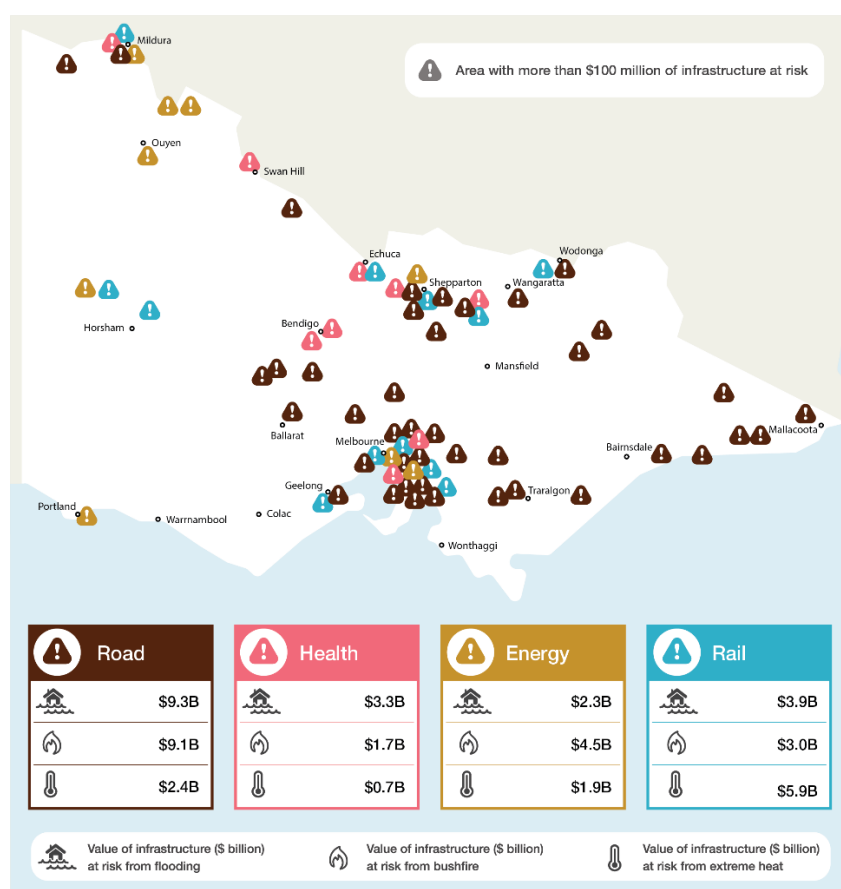
Figure 3: Areas and sectors with a large value of infrastructure at risk to climate change hazards
