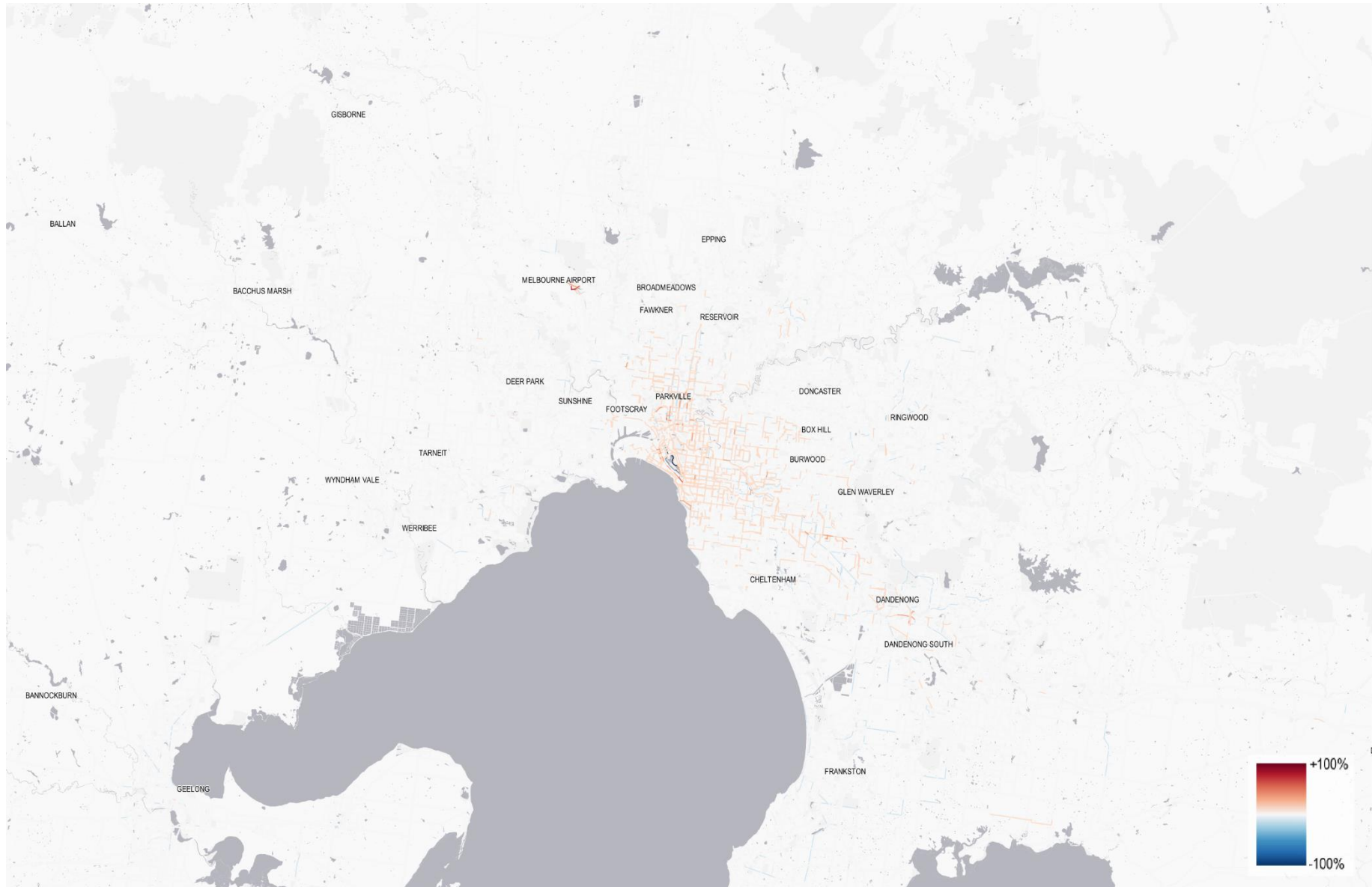
Figure 36: Morning peak volume capacity comparison, 2036 DDW vs. 2036 NDS (blue means DDW is lower)
