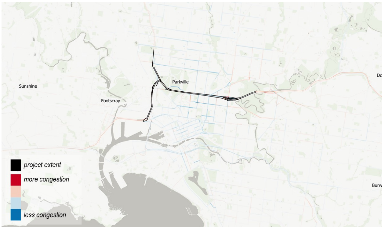
Figure D.11: Change in road volume/capacity ratio, 2051 sCCM vs. sTBC (AM period)
