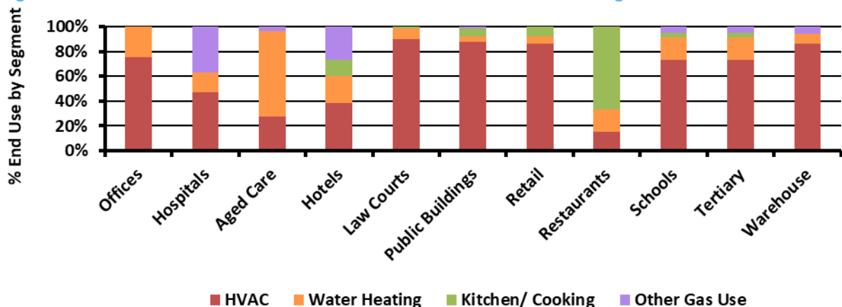
Figure 23 – Assumed Combined Gas End Use Breakdown for Commercial Segments
