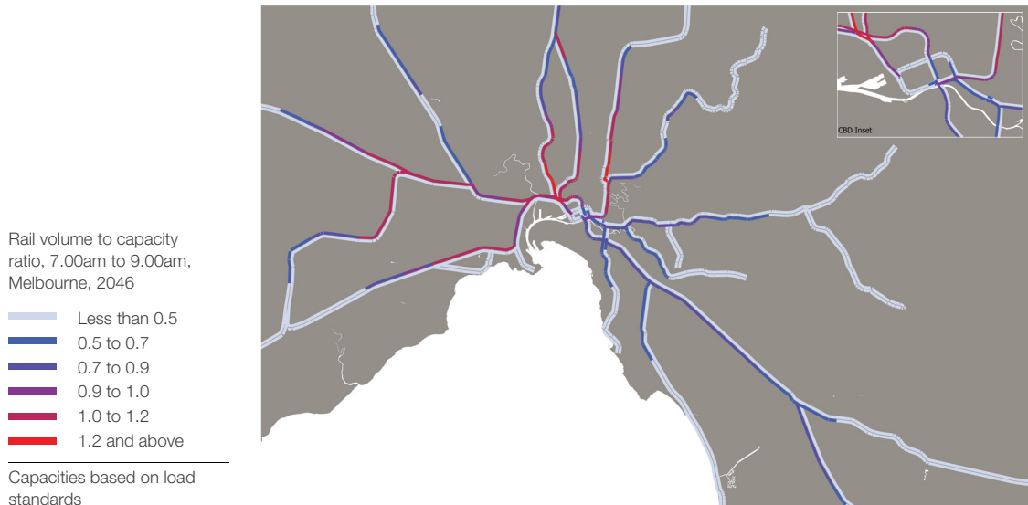
Figure 2: Even as far into the future as 2046, train lines in Melbourne's south and east are projected to have capacity during the morning peak period with only modest upgrades beyond current commitments.
