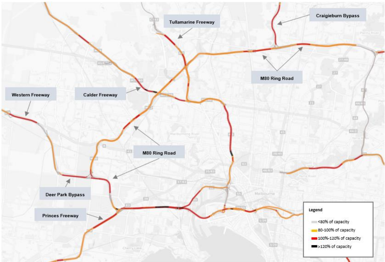
Figure 70: Traffic congestion on freeway network in 2051 (transport base case)
