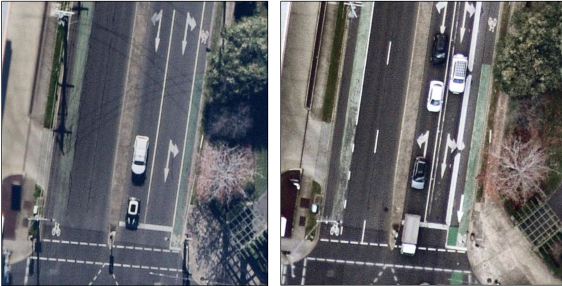
Figure 14 - Example of a change to traffic signal infrastructure to cater for separated cycling lanes
