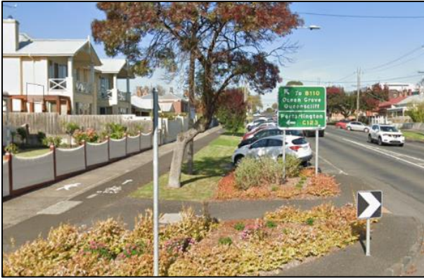
Figure 9 – Example of a one-way separated off-road facility
