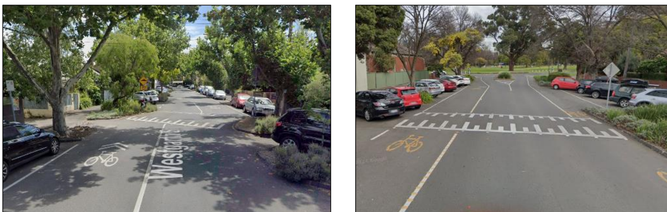
Figure 7 – Examples of bicycle boulevards, bicycle sharrows (left) and bicycle lanes (right)
