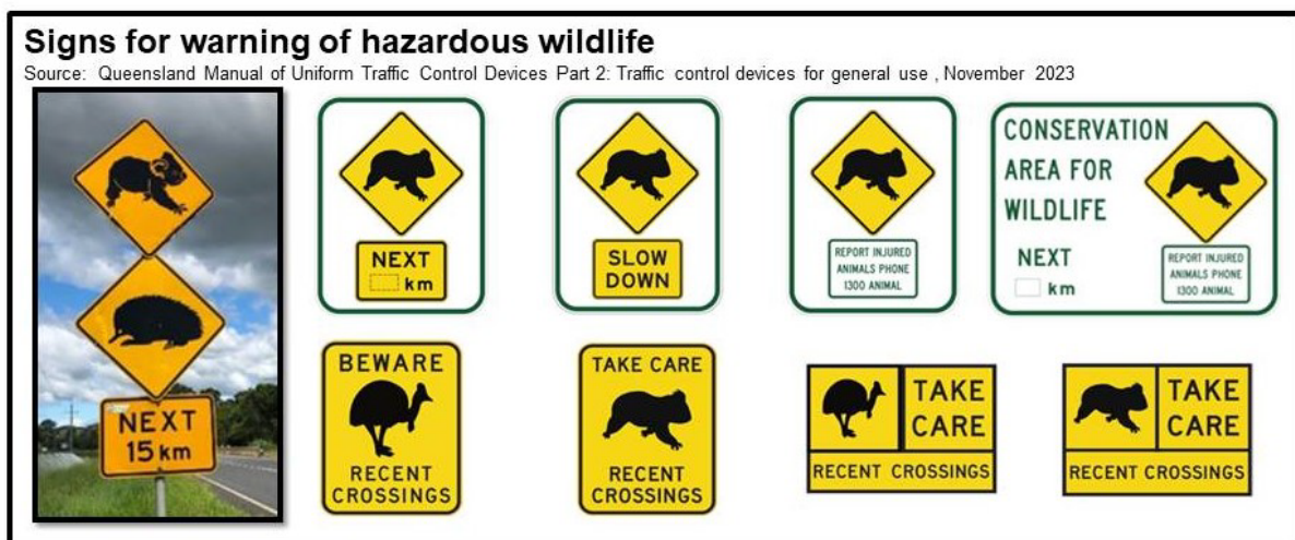
Figure 8: Queensland TMR uses a range of yellow warning signs in four categories and describes them all as ineffective for preventing wildlife vehicle collisions and inadequate for wildlife preservation. From top left: Standard; High Impact; Wildlife Conservation Area; Temporary. Source: Queensland Manual of Uniform Traffic Control Devices Part 2: Traffic control devices for general use , November 2023
