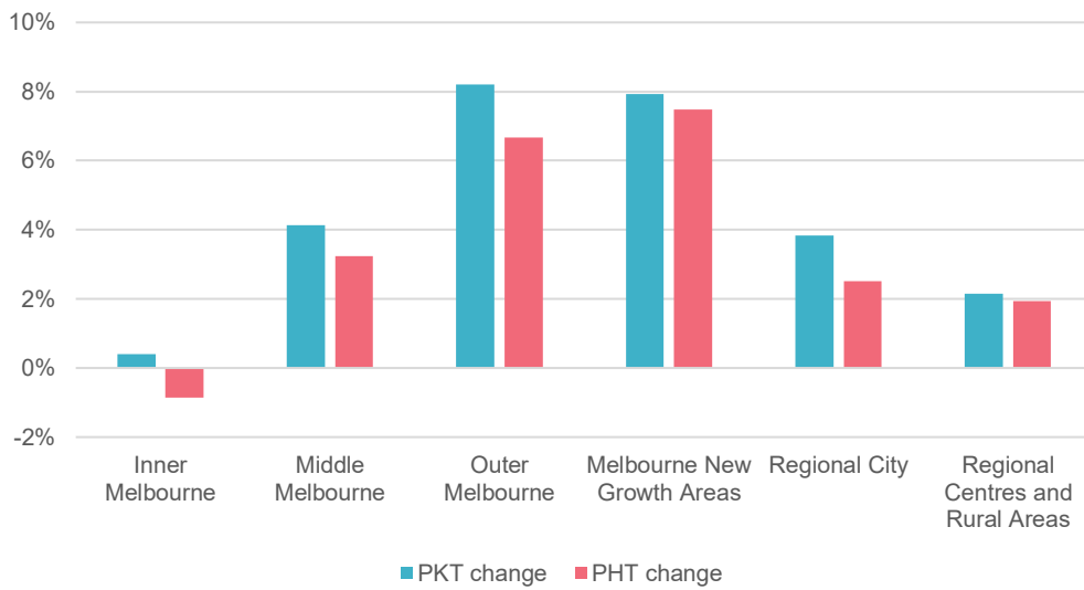
Figure 43. Change in passenger kilometres travelled (PKT) and passenger hours travelled (PHT), WFH medium vs base case, AM peak, 2036
