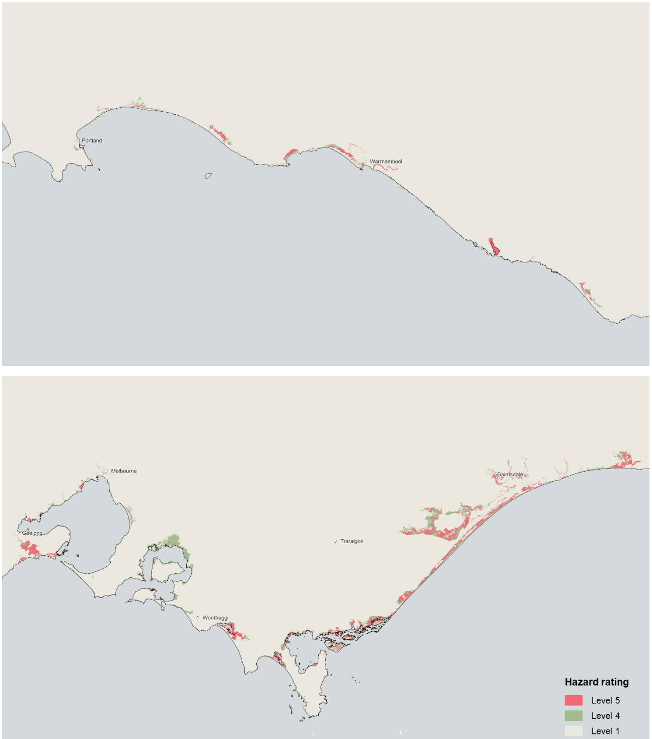
Figure 19: Coastal inundation hazard exposure map for the 47cm inundation scenario in 2070, for western Victoria (top) and eastern Victoria (bottom).
